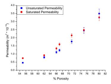
Fig. 3 Relationship between porosity and permeability for jute performs.
